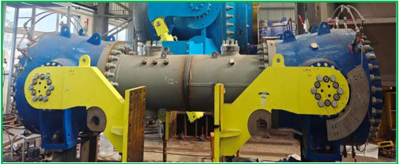
Figure Showing :- MIV Assembled with Levers and instrumentation piping
