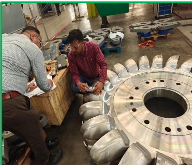
Figure: Factory Inspection of Turbine and verification of materials.
