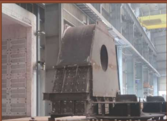
Turbine Housing fabrication
