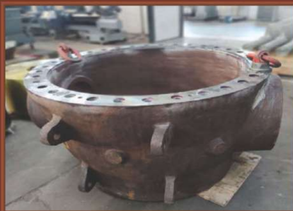
MIV upstream body casting completed
