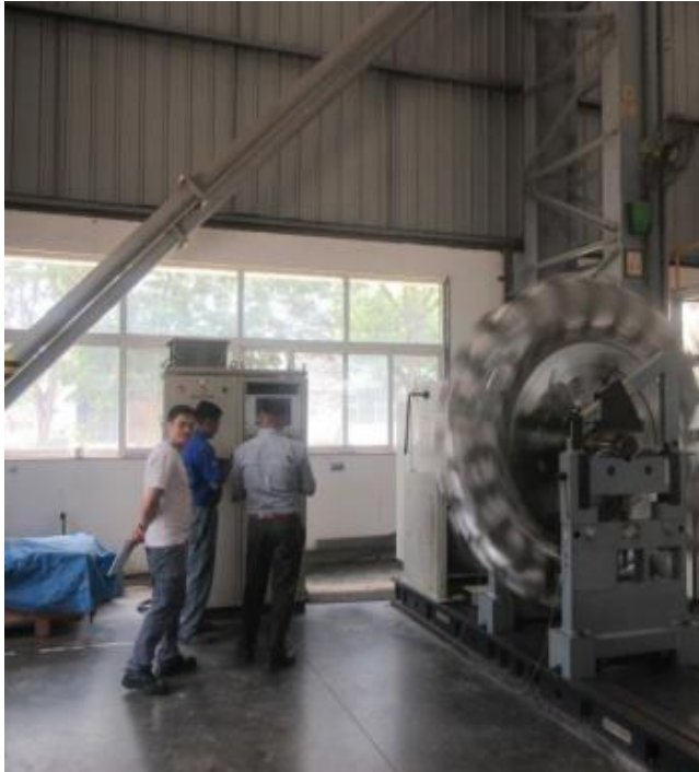
Figure: Static Balancing of Runner
