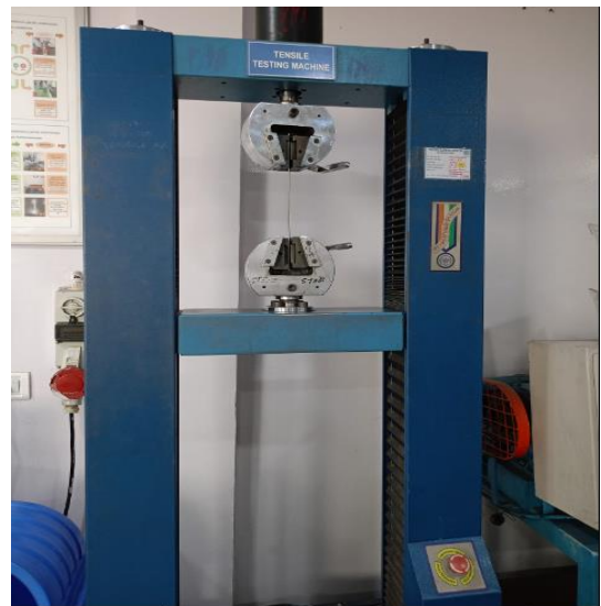
Figure: Measuring Tensile Strength of Cable Wire
