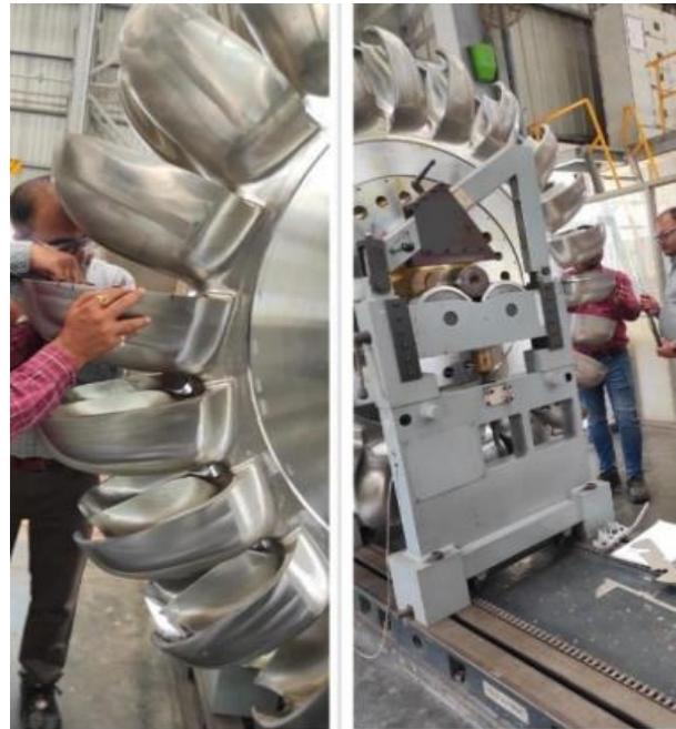
Figure: Gap measurement between template and Bucket
