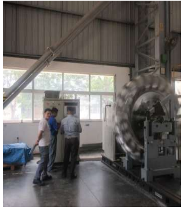
Figure: Checking of Bucket width
