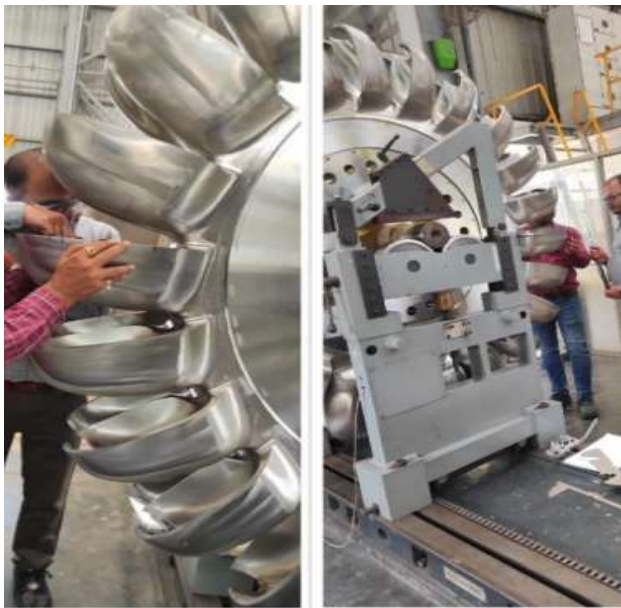
Figure: Gap measurement between template and Bucket
