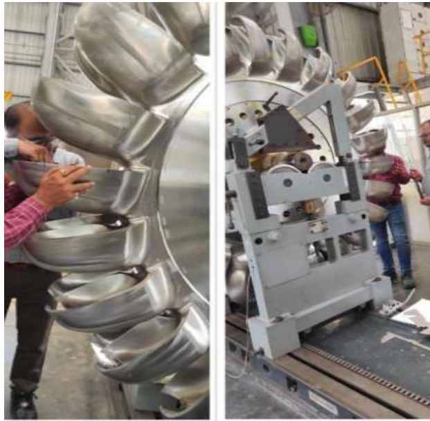
Figure: Gap measurement between template and Bucket
