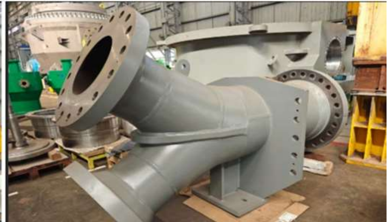
Bifurcation Pipes are ready for Dispatch.
