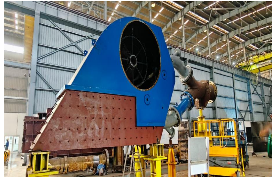
Unit 3 Turbine Housing and accessories fabrication completed and ready to dispatch
